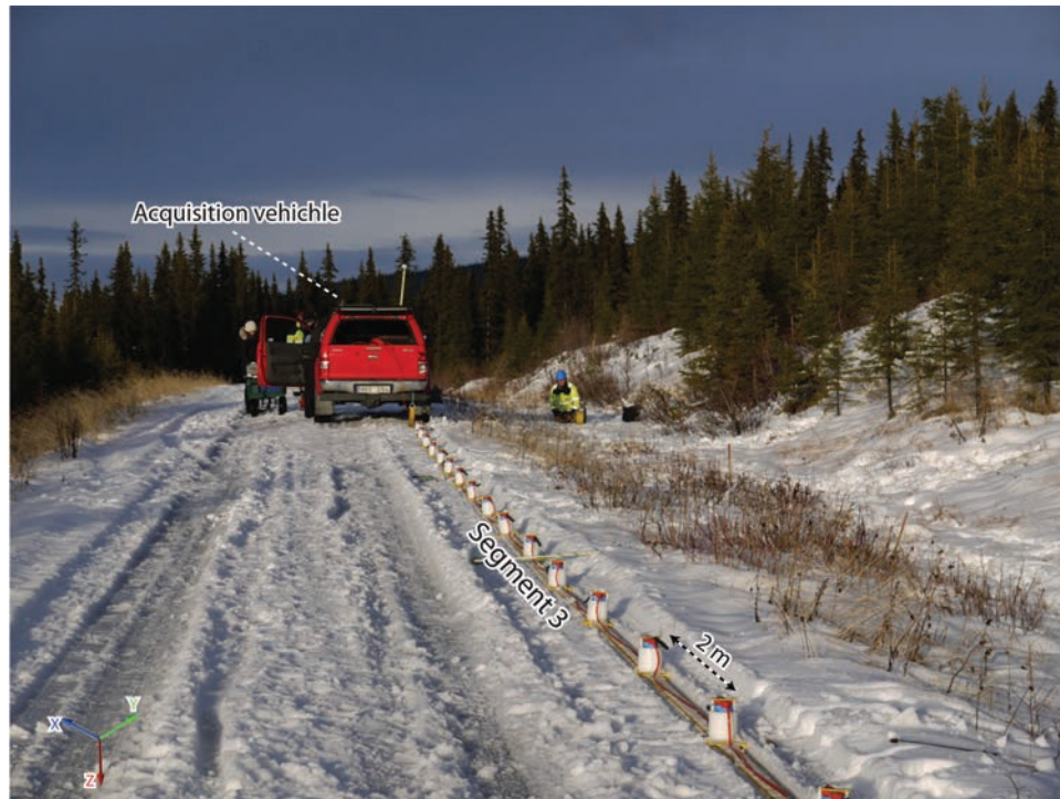
Figure 3 Photo showing the 3C seismic landstreamer system of Uppsala University used for the data acquisition in this study. Only the third segment of the streamer is seen in this photo. Three segments with a total length of about 160 m were used in this study. Note snow and frozen ground conditions during the data acquisition.
